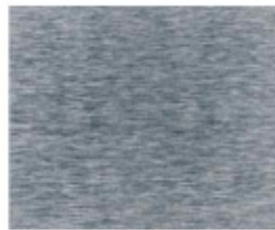
Surface finish: fine-machined, and grinded, Ra 0.2 μm
