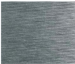
Surface finish: machined, Ra 1.2 μm
