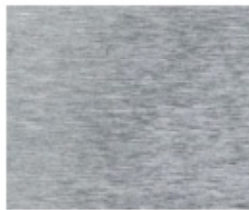
Surface finish: fine-machined, and grinded, Ra 0.4 μm
