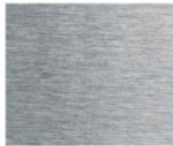
Surface finish: machined, Ra 0.8 μm
